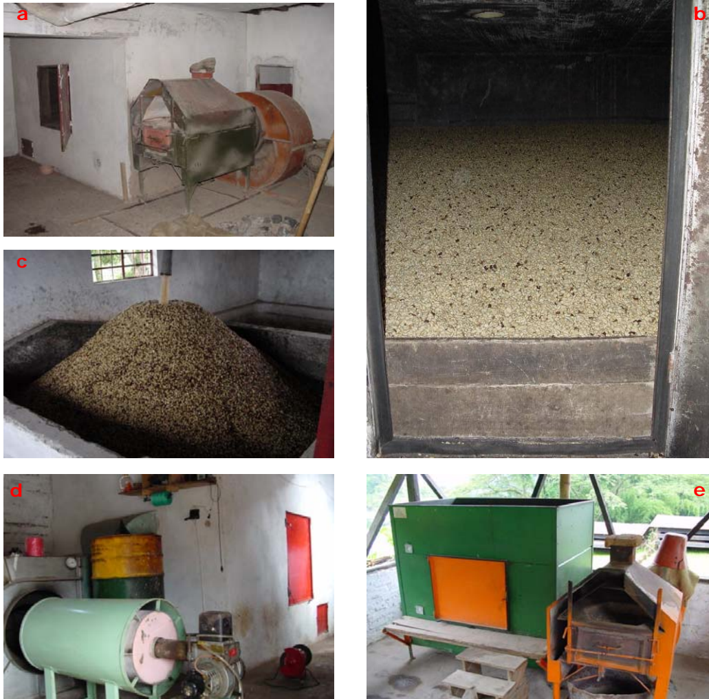
Fig. 3: Silo dryers: a. Silo dryer with a solid fuel furnace. The chamber floor is a suspended perforated steel so that the space between the chamber floor and the building floor becomes the plenum chamber or inlet manifold; b. Typically the bed thickness should not exceed 40cm - the loading port is just visible in the ceiling; c. Parchment being loaded onto the roof of a silo dryer for pre-drying; d. A silo dryer with a fuel oil furnace; e. A small silo dryer designed for smallholders. However, the farmer reported this dryer lost heat out of the sides and was expensive to operate.
