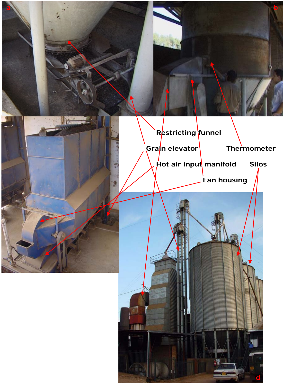
Fig. 1: Vertical dryers: a. The flow-restricting funnel is a fixed orifice and the elevator runs at a fixed rate thus residence time in the drying column is fixed at a given load; b. Ambient and heated air is mixed at the input manifold and the input temperature is adjusted to the manufacturers recommendation; c. Both cubic and circular cross sections are available in this approach to drying; d. Dryers at exporters and large traders, as opposed to farmers, are of a different scale.
