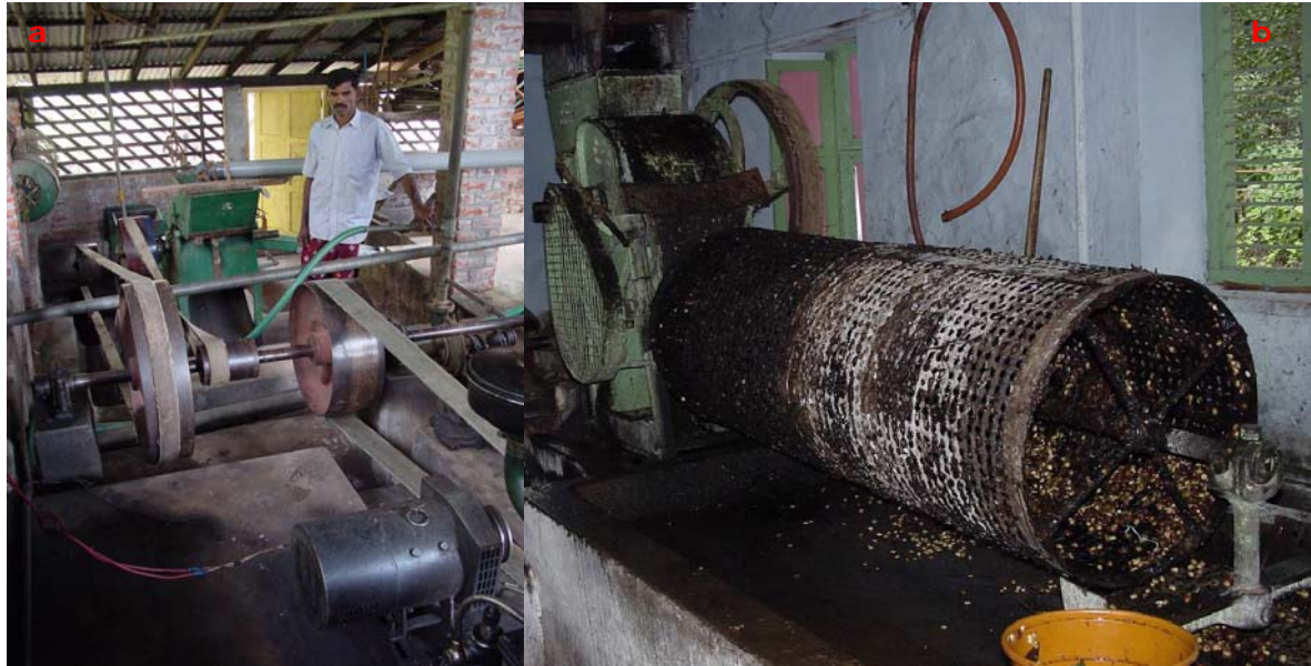
Fig. 4: a. Belt drives isolate the motor from water but unprotected belt drives provide a hazard to the operators; b. Corrosion of the steel sieve due to prolonged contact with coffee mucilage is clearly visible.
