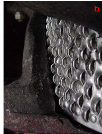
Fig. 1: Three current pulping systems: a. Disc pulper; b. Drum pulper which can be either horizontal or, as here, vertical; c. strip harvest pulping system omitting the lavador which separates floating coffee.
