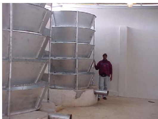
Fig. 3 - Metal silos for green bean storage with aeration systems in an enclosed storage area
